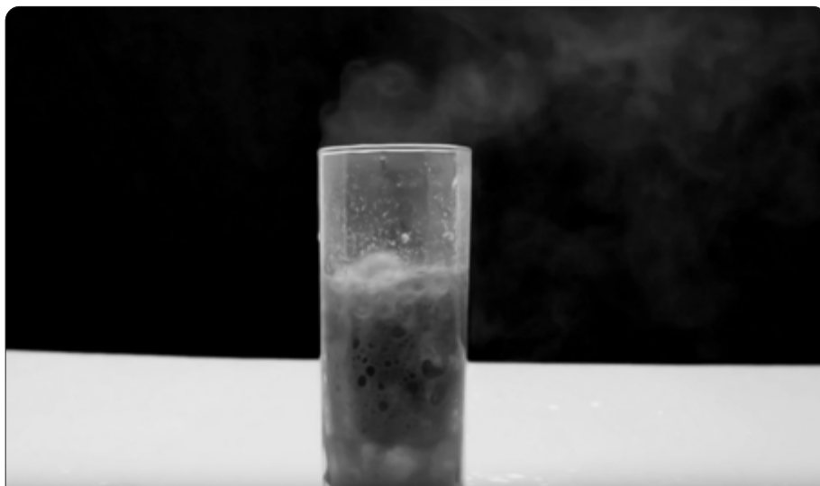
Image 101. The reaction between an acidic toilet cleaner and a hypochlorite bleaching powder releases chlorine gas.
