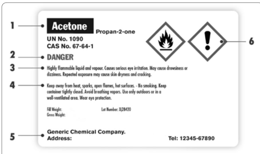
Image 93. A warning label that is compliant with GHS guidelines. (1) Product identifier: Acetone (the common name), Propan-2-one (the preferred IUPAC name), CAS NO. 67-64-1, and UN 1090. The names used on the label should be identical to the ones used in the SDS (2) Signal word: Danger. (3) Standardised Hazard Statements. (4) Precautionary Statements. (5) Contact information of the manufacturer. (6) Pictograms.
