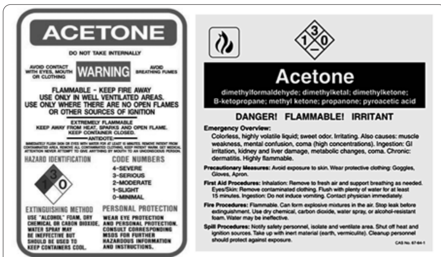
Image 95. Warning labels for acetone. Neither is compliant with GHS recommendations.
