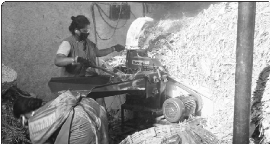
Image 65. ♻ Kokila uses 4242 rated TYPE DW gloves when she operates the shredder. Notice that she uses a stick to push garden waste into the machine. The glove will not protect her from injury from the shredder! It protects her hands from sharp splinters. She keeps a pair of TYPE WW gloves in her overalls for handling wet waste. She is wearing ear-plugs, and eye protection.
