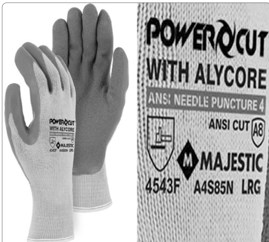
Image 58. Glove rated EN388 4543F and ANSI A8, appropriate for jobs that present extreme cut and puncture hazards. These gloves are relatively expensive, costing more than ₹800 for a pair. Participants often ask if e-waste workers should use such gloves if they handle glass—such workers often deal with fragile incandescent and fluorescent bulbs. Selection of PPE depends on the job, and only after engineering controls have been implemented. Can the hazard be reduced by the use of tools and jigs? If so, that is the appropriate recommendation.
