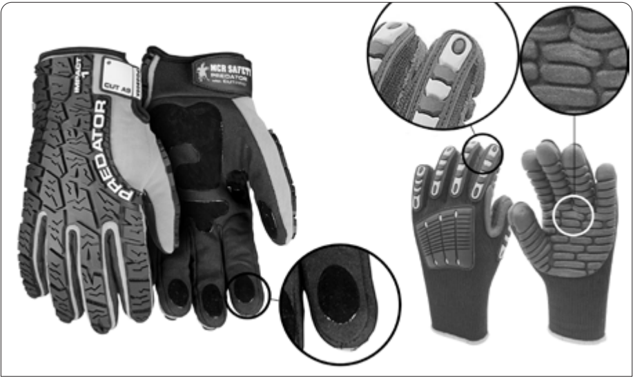
IMAGE 61. TYPE S gloves (L) with impact-protection pads on the back of the hand, and leather grip-pads on the fingers and palm and (R) with shock-absorbing pads on the palm and fingers. These pads reduce the fatigue and muscle-tension when working for long hours with power tools, such as impact drills and demolition hammers. Safety, then comfort should be the criteria to determine whether these special-purpose gloves are appropriate. Some workers prefer TYPE GP leather gloves for such jobs; others prefer a cushioned glove. (Photo credit: https://workwear.co.uk )
