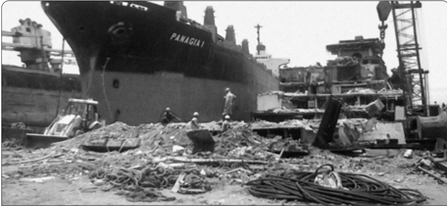
Image 63. A ship being dismantled for scrap in Alang, India. Though ship-breaking does not usually come to mind when discussing Solid Waste Management, what else is ship-breaking but recycling at an industrial scale? SWM workers in this sector are exposed to high-risk cut, puncture, impact, chemical, fire, and electrical hazards. (Photo credit: Anil C. Patel, Wikimedia Commons.)
