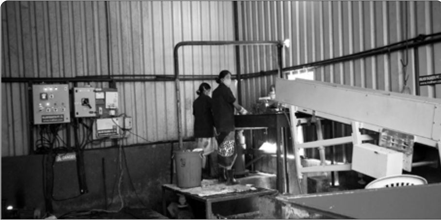
Image 128. SWM workers at a fully mechanised biogas plant wearing appropriate SRC+s4 boots, properly fitting jackets, masks and TYPE WW nitrile gloves. When loading the conveyor, they wear PVC aprons (kept hanging on pegs just out of sight on the right) Both are trained to operate all the machinery in the plant. ♻
