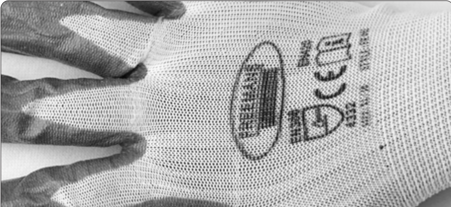
Image 67. Beware of fake stamps and markings. This glove is made from polyester and is coated with a thin, uneven layer of recycled PVC. It cannot possibly achieve its rated safety performance of 4332. It is a cheap imitation of a rated glove made by a reputed company. It is possible that this glove may be a factory reject—perhaps a lower-rated glove was stamped incorrectly—however, the poor fit and quality of printing suggests otherwise. Poor quality prints are usually found only on fakes. See IMAGE 48 → [126] for an example of good printing quality.
