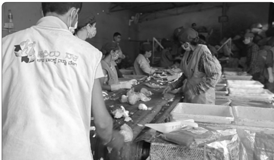
Image 142. ♻️ Workers at the mixed-waste sorting station in ELCITA are able to work without fatigue for longer because their sorting workstations are ergonomic and the sorting procedures are properly designed — they use a conveyor, workers use appropriate gloves depending upon what they sort, they do not need to bend, notice that their hands remain at waist level at all times, even when transferring sorted material to the bins.
