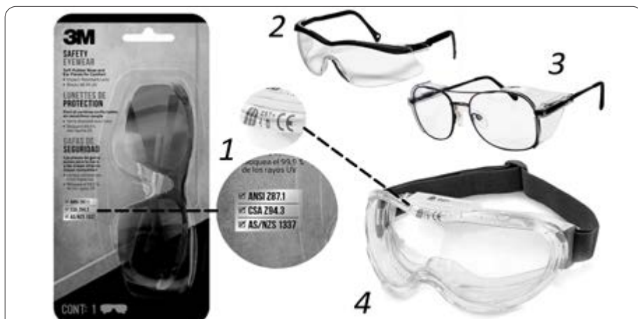
Image 122. (1) Look for a z87.1 stamp or mark embossed on the lens or on the packaging. (2) Safety glasses; (3) Side-shields attached to prescription glasses. (4) Safety goggles. Premium products have a durable scratch resistant coating, and offer 100% protection from uv light.
