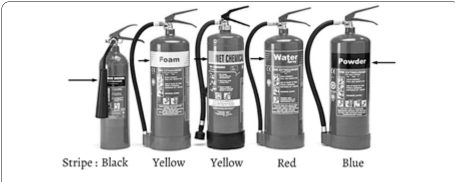
Image 130. Different types of fire extinguishers. A dry-powder model (identified by a blue stripe on the body) is suitable for A-, B-, and C-CLASS fires.
