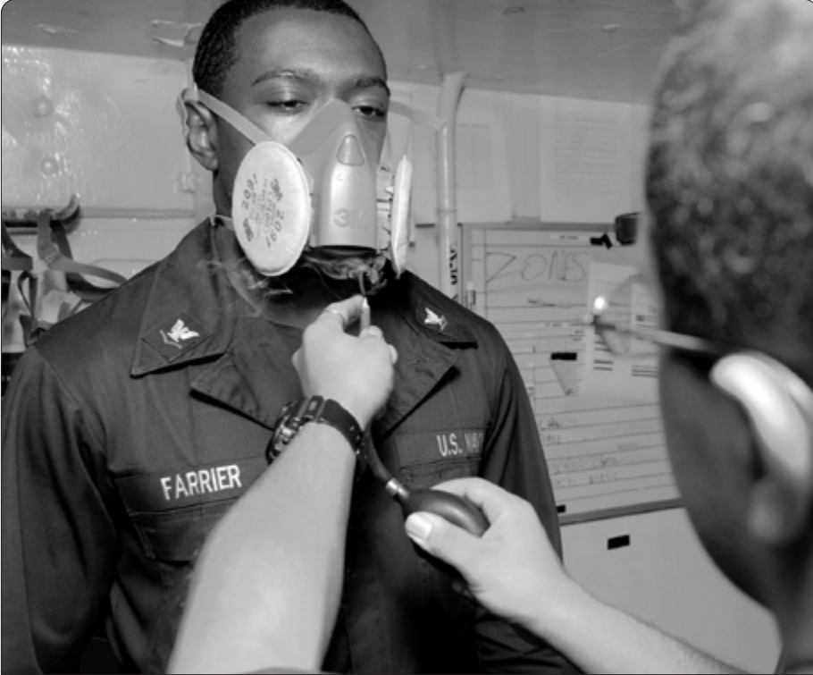
Image 108. Qualitative fit test of a respirator. The tester is holding a bulb filled with an irritant vapour that induces an involuntary cough reflex in the wearer. The use of a diffuser is more convenient even though the test is not precisely repeatable. (Photo credit: Daniel J. Meshel.)
