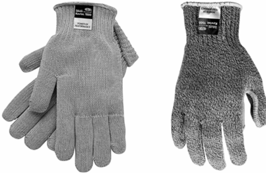
Image 57. (L) TYPE GP safety glove made with knitted 7-gauge pure Kevlar® threads. It may look like a plain, knitted cotton glove, but its cut-protection is five times better; it is lighter and dries faster. (R) A glove made with 7-gauge Kevlar® and stainless steel threads.
