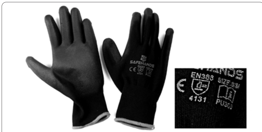
Image 48. Generic, commonly available TYPE DW glove with polyurethane coating. It has an EN388 rating of 4131. What do these numbers mean?
