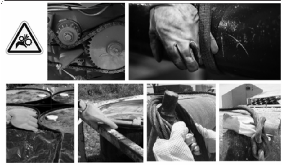
Image 71. Nip-points in machinery (Top row, from left to right) Nip-point hazard pictogram; exposed chain-transmission in wood-chipper; canvas winch-line; (Bottom row, from left to right) closely-spaced heavy objects such as drums; the space between fences and drums, crates and so on; bridal and winch lines, in general, should always be treated as pinch-hazards; PPE does not protect against pinch hazards.
