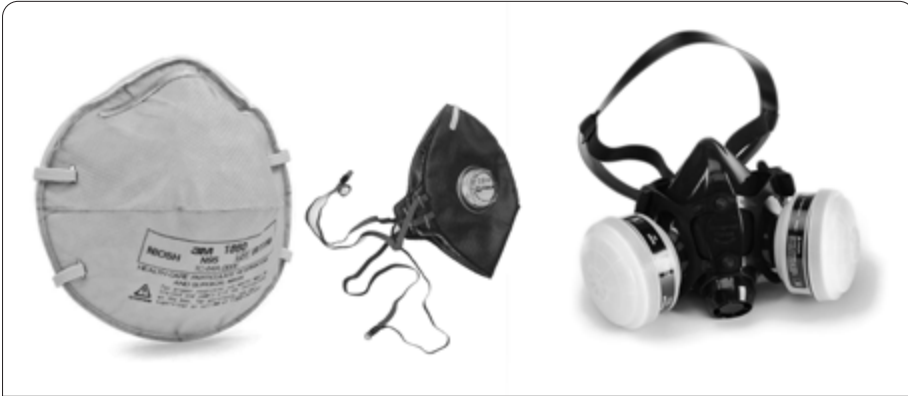
Image 102. Options for respiratory protection. (From left) Disposable FFP-style mask rated N95 with a fibre filter; washable mask with fibre filter cartridge rated EN149-FFP2 and an exhalation valve; half-face respirator with replaceable cartridges.
