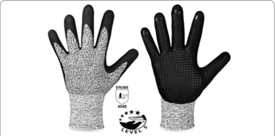
Image 55. ♻ Back and front of a TYPE DW Dyneema® fabric glove with nitrile coating. Its palm and fingers are textured with large, soft dots. This glove has an EN388 rating of 4540 and can be used for handling sheets of glass and metal.
