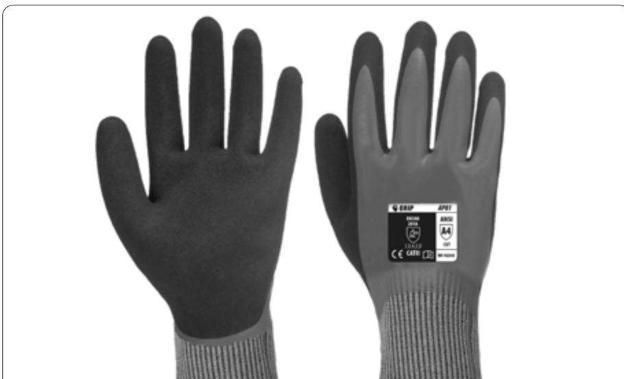
Image 77. Fully coated TYPE DW gloves, rated EN 3434D. These are designed for wet-work; they have a comfortable inner lining that absorbs moisture and the nitrile texture offers excellent wet grip. However, they are more expensive than nitrile TYPE WW gloves, which do not have an inner lining. This glove is a catch-all recommendation for SWM workers who process wet-waste.
