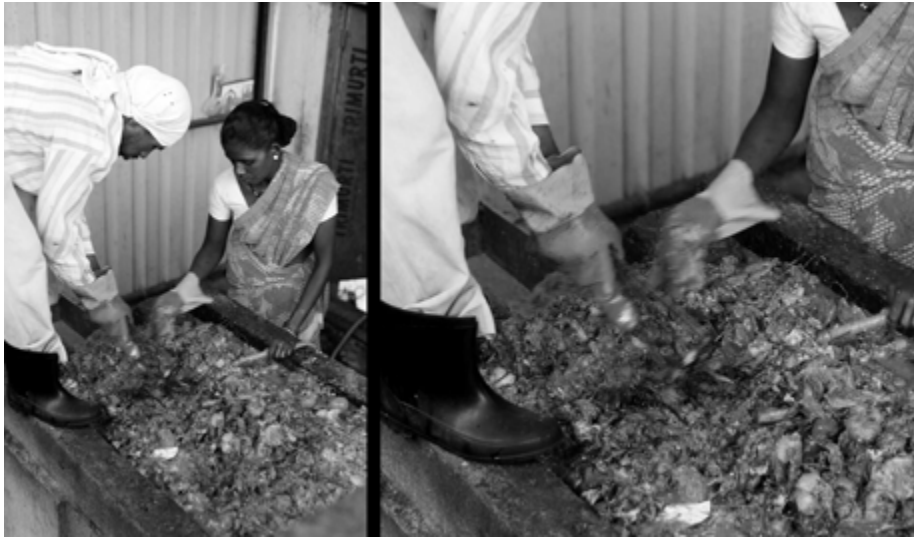
Image 78. (Slide 2) Workers at a biogas and compost facility. Both are wearing ill-fitting nitrile dish-washing gloves and gum-boots. Clearly, their usage of PPE does little to address the many hazards in the workplace. Identify the hazards. Discuss how the safety of these workers may be improved using the Hierarchy of Hazard Control.
